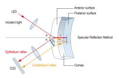
CCT (Central Cornea Thickness) Measurement Concept
